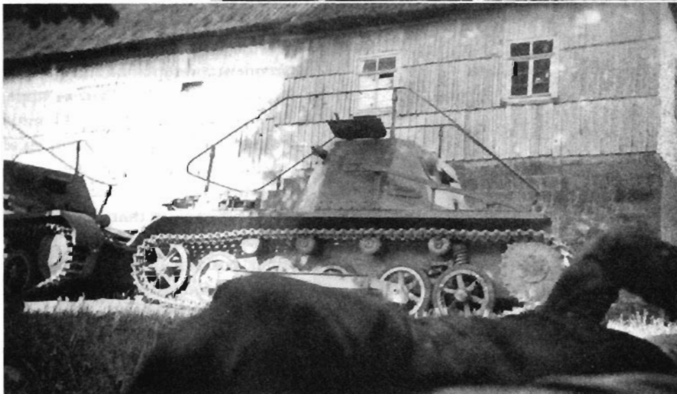
Early command and control vehicles were based on the chassis of the Panzer I. These versions are the kleiner Befehlspanzer I, Ausführung B.
