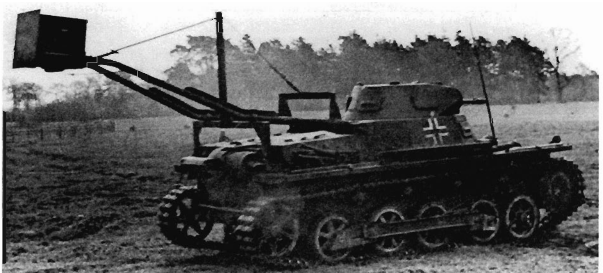
The Wehrmacht had demolition-carriers and radio-controlled demolition tanks for blowing up obstacles under enemy fire. In these two photographs we see the Ladungsleger auf Fahrgestell Pz.Kpfw. I which was only used to mixed effect early in the war.
