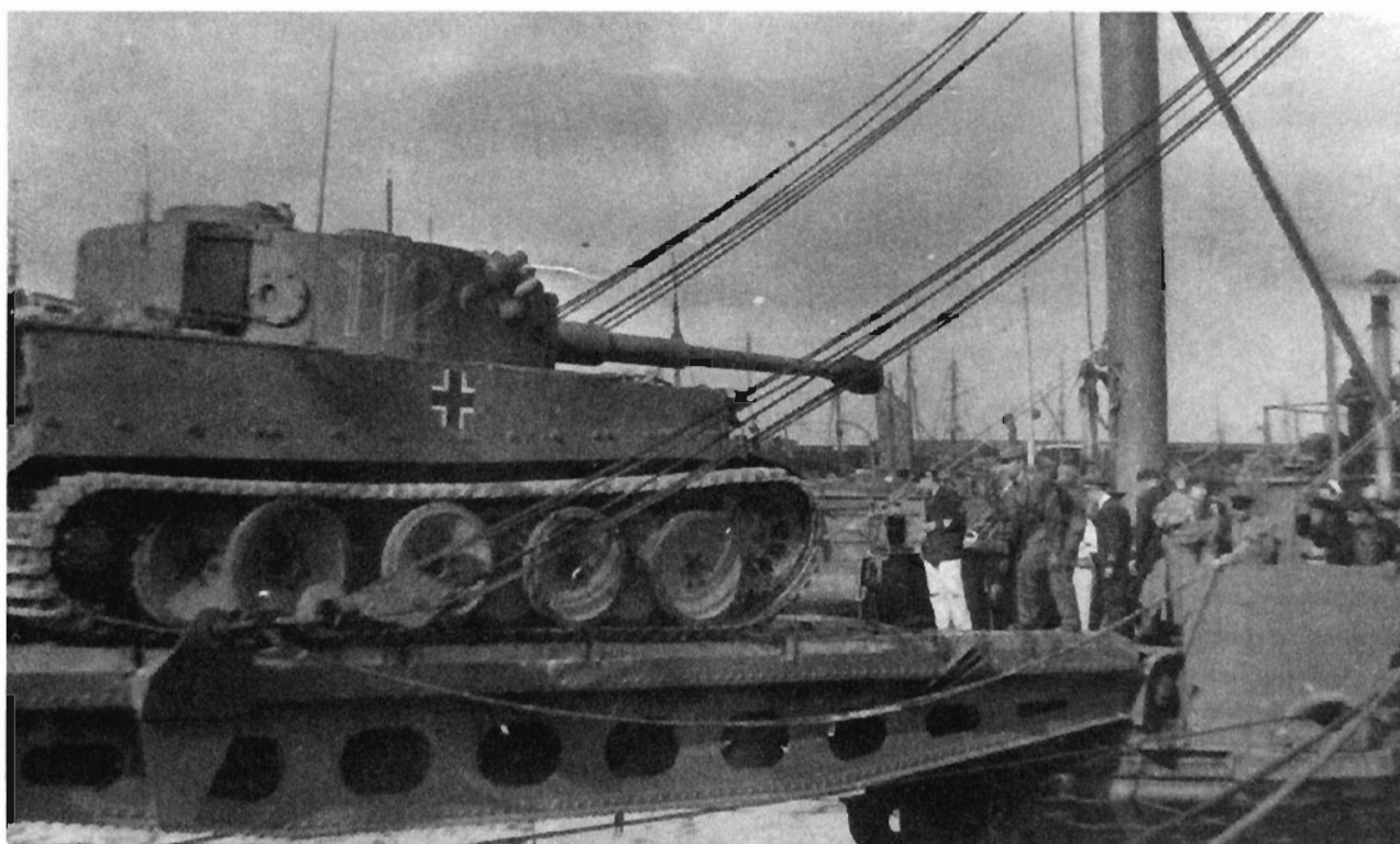
With a roll-on, roll-off ship, the unit vehicles drive on ramps under their own power directly into the holds. Securing and unloading them is also relatively simple, particularly if the trip is a short one. HARTMANN
