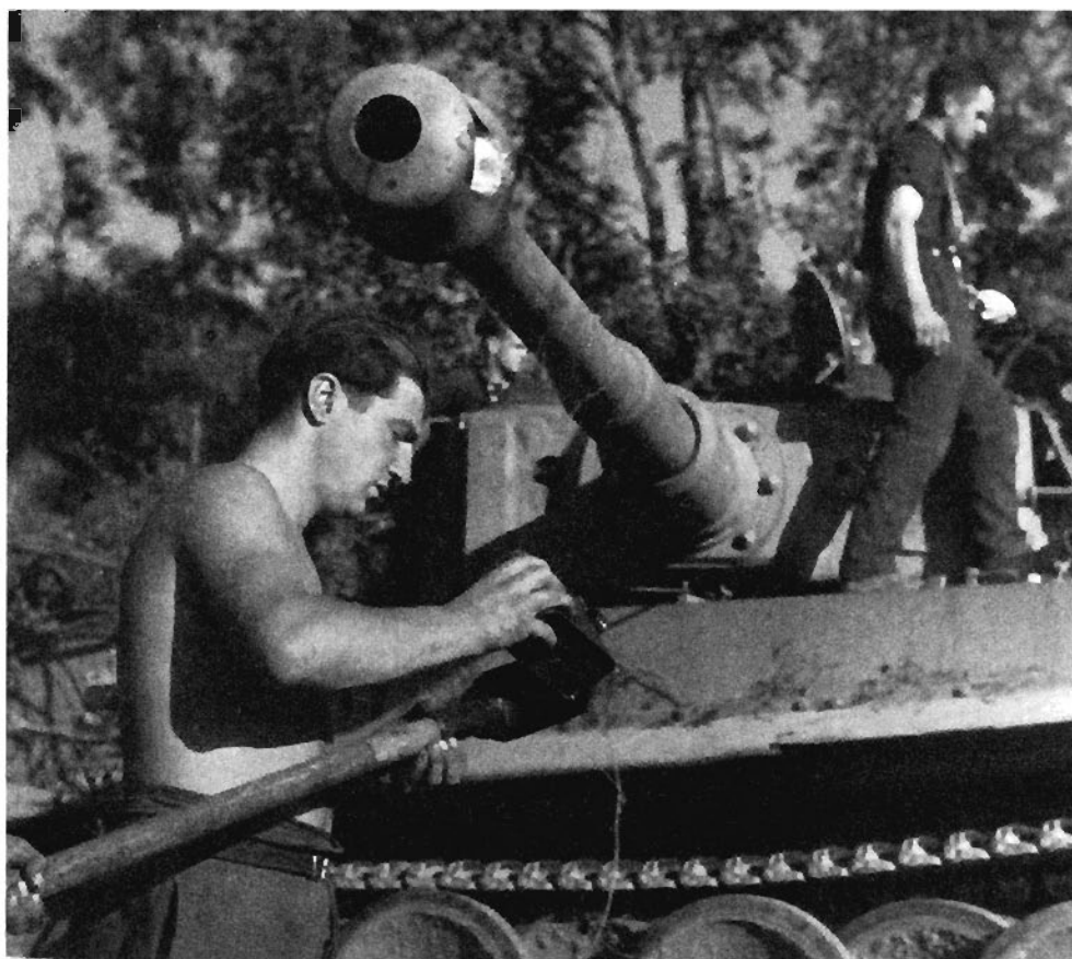
Cleaning the gun barrel is a requirement after the gun has been fired. To do that, the stowed cleaning rod is assembled and cleaning/oiling attachments are placed on the end. Swabbing the barrel is a crew effort and requires a lot of work to do it properly.
