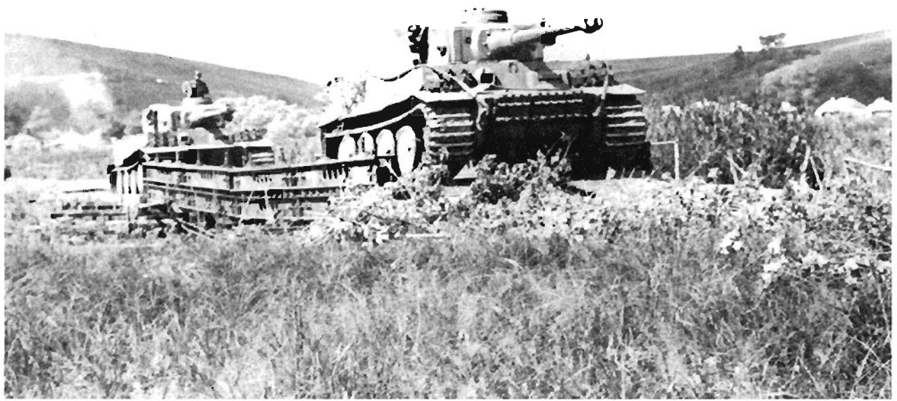
Small water courses and cuts can be crossed with provisional military bridges. They can be brought forward in minutes, particularly when transported on a bridge-laying tank.
