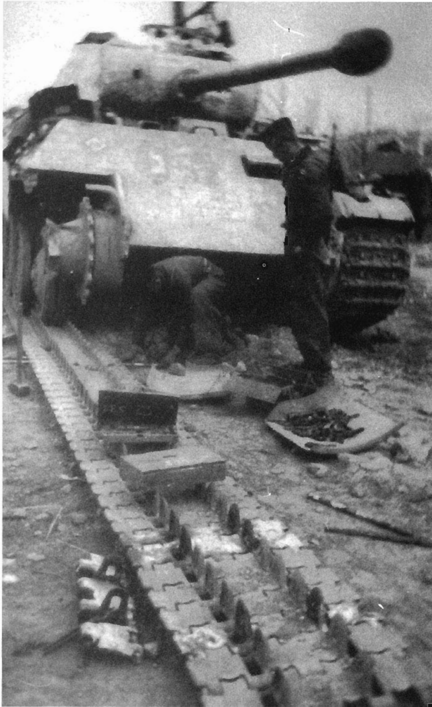
Often—all too often—the tank crew has to work on running gear and tracks. The repair and maintenance platoon only helps in exceptional cases.
