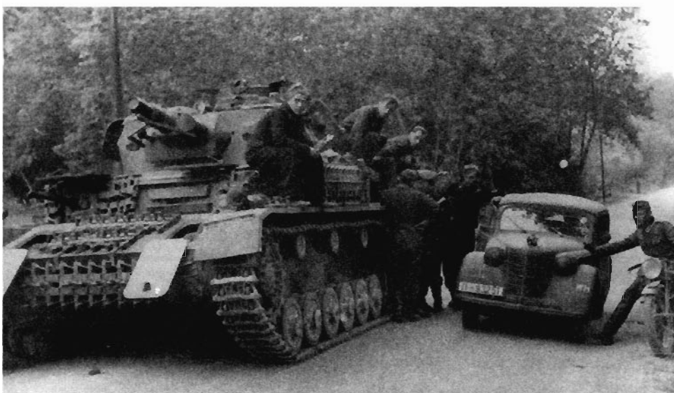
Vehicles with breakdowns, such as the Panzer IV with damaged steering brakes in this picture, are not allowed to block the march route. The trail officer at the end of the march column stops at the damaged tank, determines the cause of the breakdown and takes additional action. KARL HEINZ MÜNCH
