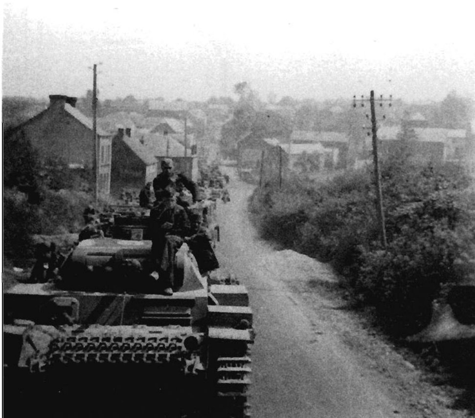
Whenever possible, maintenance halts were frequently called (about every 30 to 60 minutes), particularly to check the running gear for damage. Because of the limited driving range of the vehicles, these halts are also used to refuel.
