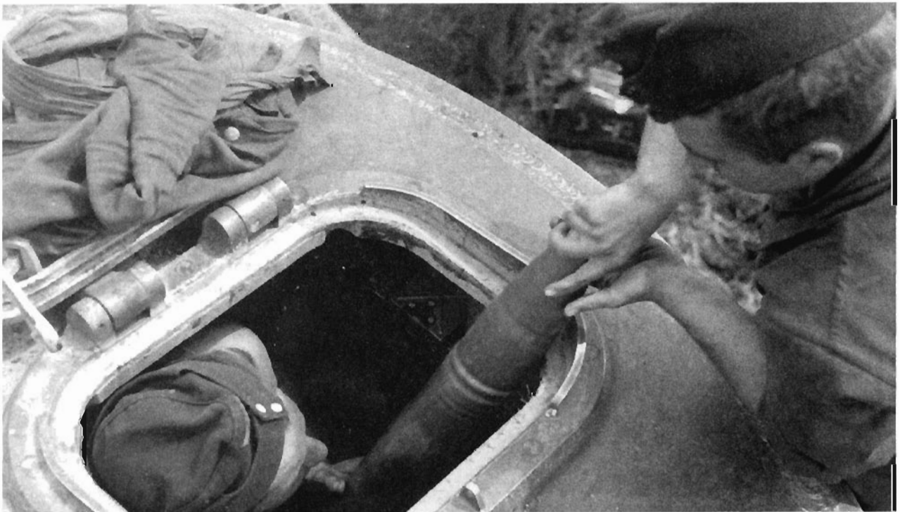
The ammunition is removed from the containers and passed up by a crew member from down on the ground. The rounds of fixed ammunition are passed in through one of the hatches and stowed away in the racks.
