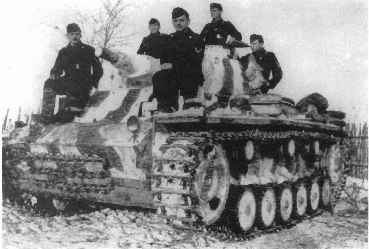
If the tank is employed in snow-covered terrain, the crew has to use a whitewash mixture to produce large, irregular blotches and stripes.
