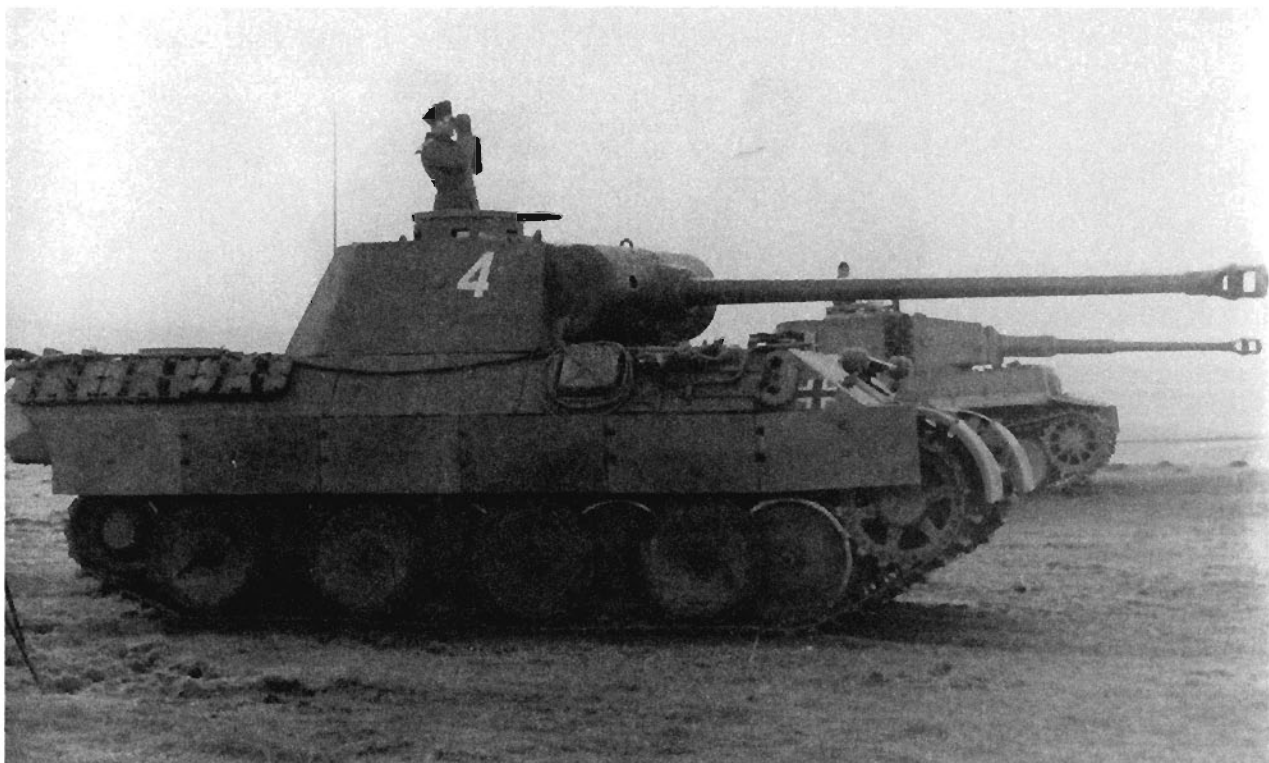
The essential foundation for the tank soldier is mastery of tank gunnery. In contrast to automatic weapons, the emphasis has to be on precision and on securing a hit with the first round. Shown is a gunnery comparison between the prototypes of the Panther and the Tiger.
