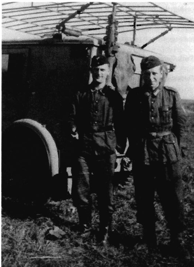
Far-reaching radio communications above the company level could not usually be established on ultra-short radio-wave sets. For that purpose, special short- and medium-wave radio vehicles were also employed as illustrated here with the Funk-Kraftfahrzeug 17.
